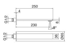
**CONSTRUCTION:** 316 Stainless Steel **PRESSURE:** Mains Pressure Only
