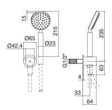
**CONSTRUCTION:** 316 Stainless Steel **PRESSURE:** Mains Pressure Only
