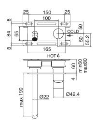
**CONSTRUCTION:** 316 Stainless Steel PRESSURE: Mains Pressure Only
