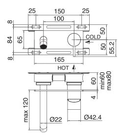
**CONSTRUCTION:** 316 Stainless Steel PRESSURE: Mains Pressure Only
