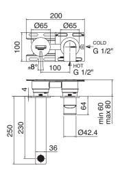
**CONSTRUCTION:** 316 Stainless Steel **PRESSURE:** Mains Pressure Only
